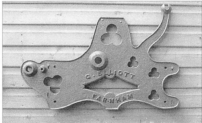
Fig. 3 One of a pair of side panels from a hop-compressing machine, bearing the name of G. Elliott, Farnham. (Photograph by Glenys Crocker.)
