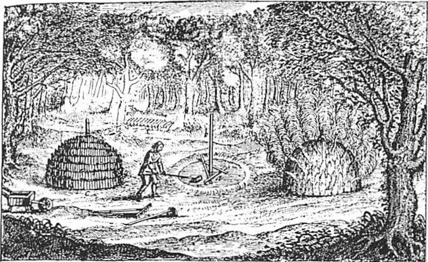
Fig. 2. Three Stages in the Traditional Method of Making Charcoal in clamps, as illustrated in John Evelyn's Sylva . (Courtesy of Surrey Archaeological Society).
