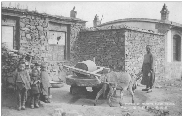
The flour was removed from the lower stone by the farmer walking round using a brush to clear the flour.
