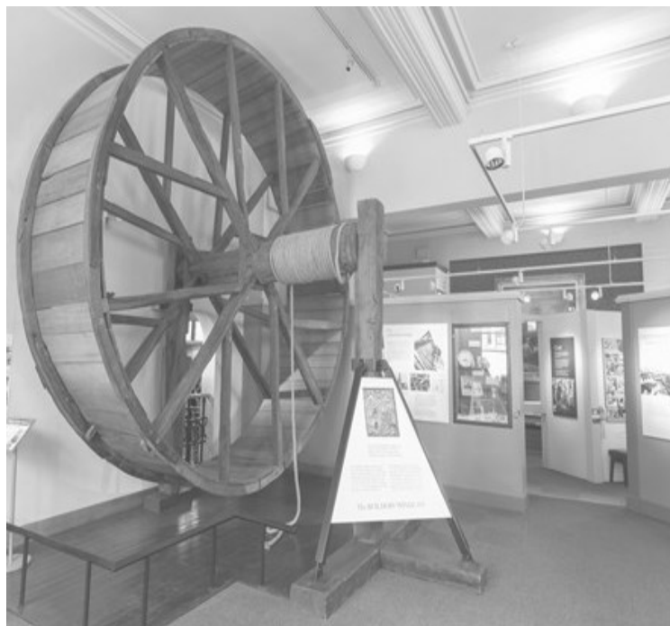
The medieval builders' wheel, was used over 600 years ago in the building of the famous Crooked Spire church.
