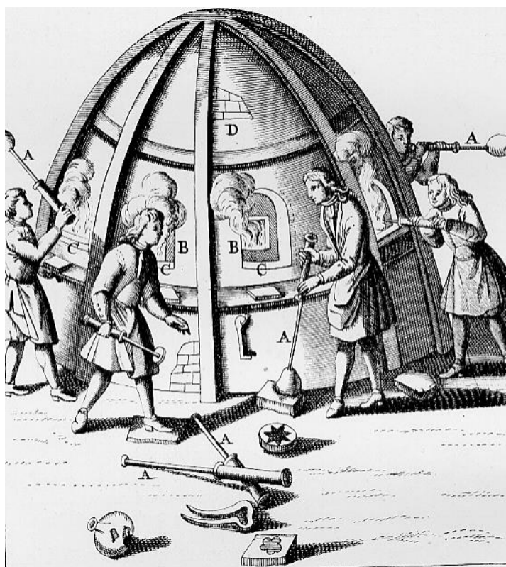
17c glass furnace; showing blowing-irons, moulds and a broken wine bottle
